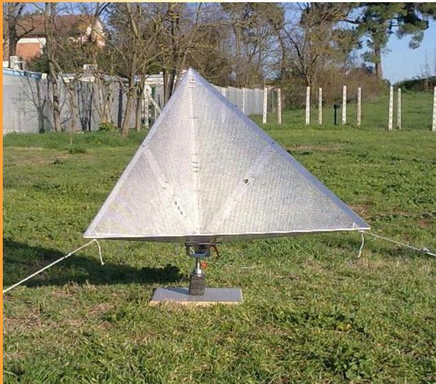
*The first prototype of Corner Reflector*
